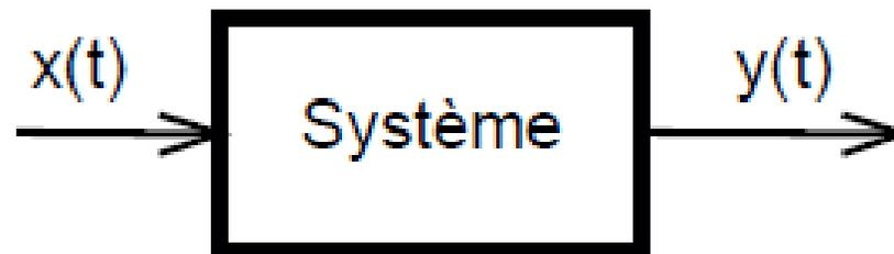
$$a_n \frac{d^n y}{dt^n} + \dots + a_0 y = b_m \frac{d^m x}{dt^m} + \dots + b_0 x$$
